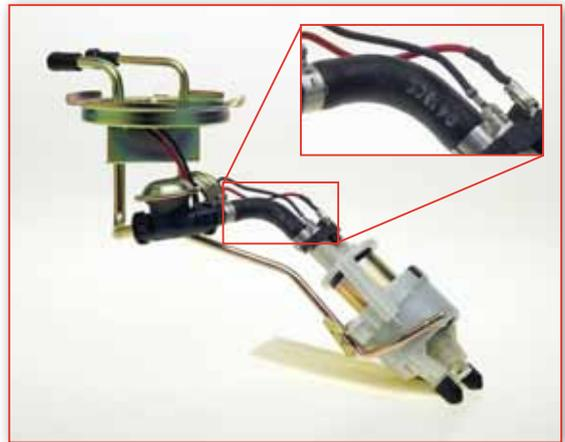
*Unfortunately, too many in-tank fuel pump repairs improperly use ordinary fuel line hose for the pump-to-valve connection.*
