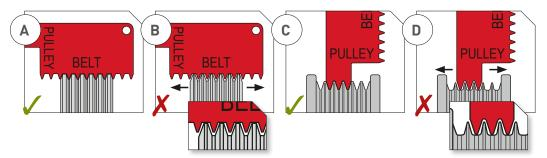
The Gates ABDS wear indicator results indicate an approximation of the material loss from the belt, which should be taken into consideration with other factors – such as mileage, operation conditions, and the condition of other components of the accessory drive. You should rely on your experience as a professional technician when making repair recommendations.
